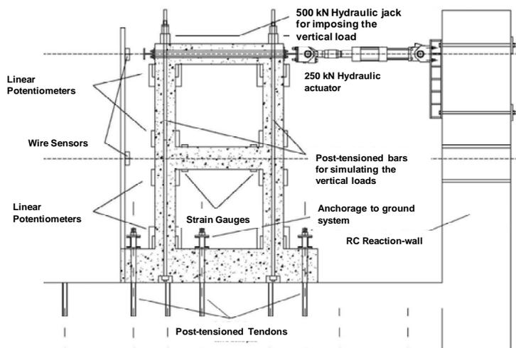
Figure 3 – Test specimen and experimental setup
