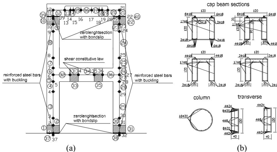
Figure 9 (a) Finite element model scheme. (b) Element sections (actual dimension and reinforcing steel).
