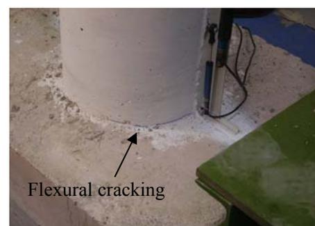
Figure 8 – Cracks at the base of a column
