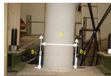
Figure 4 – Displacement transducers
