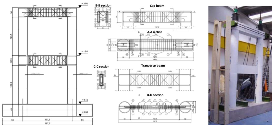
Figure 2 – Test specimen and reinforcement details
