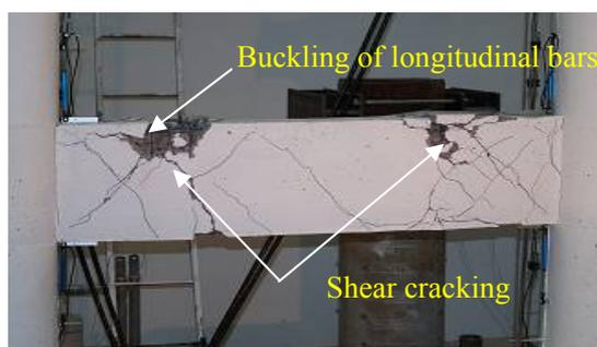
Figure 7 – Shear cracking pattern of the transverse
