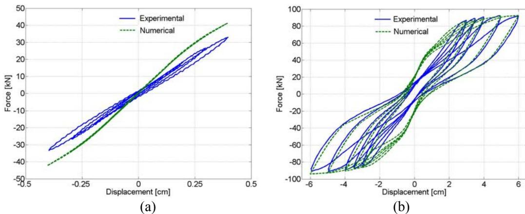
Figure 10 (a) Experimental and numerical cyclic response  $D_c = 0 - 0.4$  cm. (b) Experimental and numerical cyclic response  $D_c = 3.0 - 6.0$  cm.
