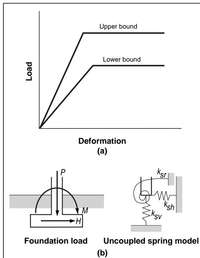
**Figure 4-1** (a) Idealized Elasto-Plastic Load-Deformation Behavior for Soils
