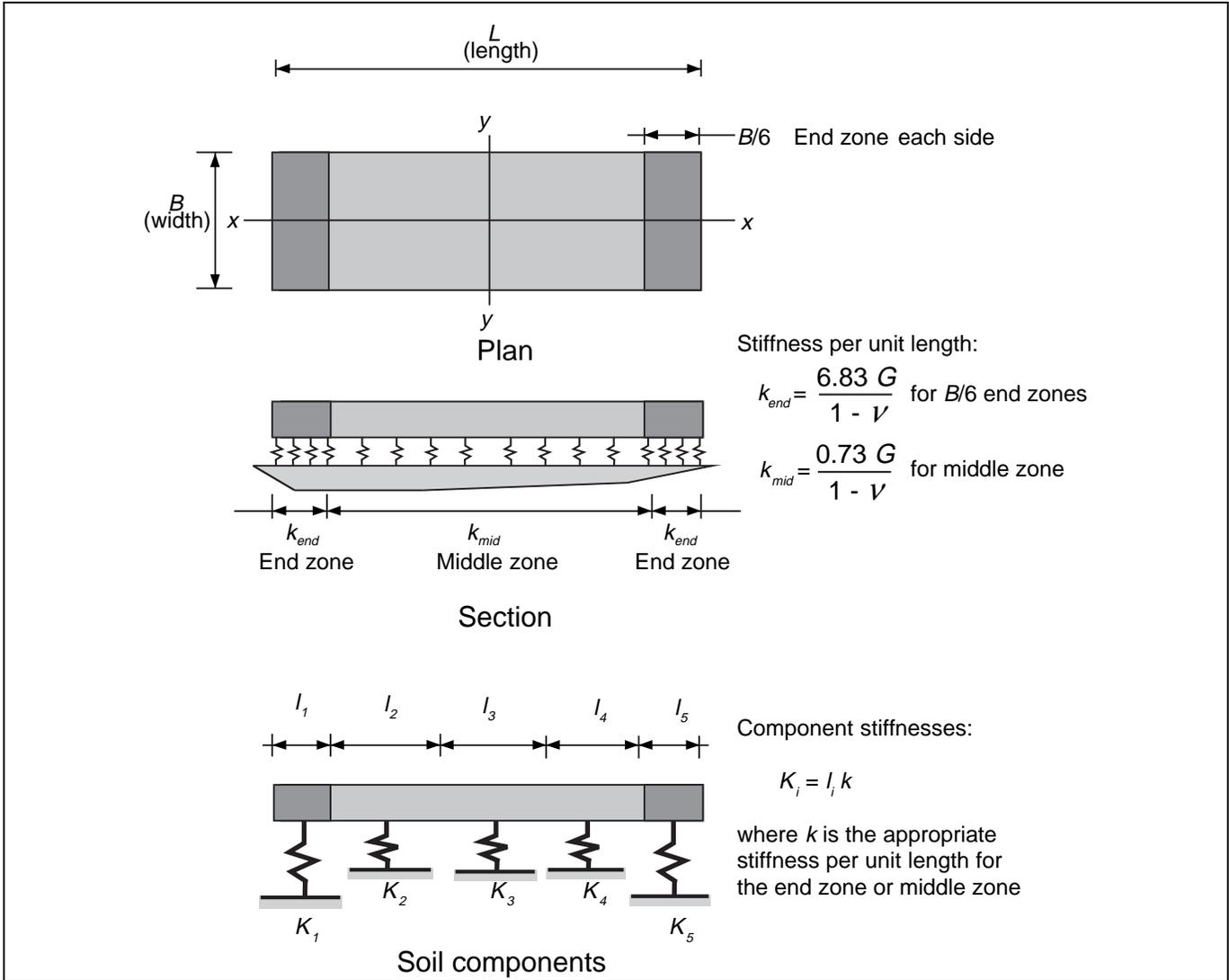
Figure 4-5 Vertical Stiffness Modeling for Shallow Bearing Footings
