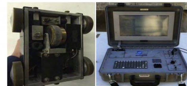
(b) IE scanner and DAQ PC
