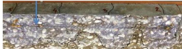
Chloride ingress in a beam with bending cracks
