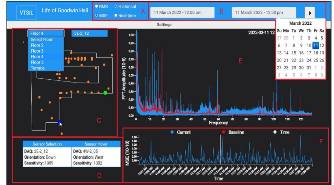
Fig. 4. Dashboard showing the frequency spectrum (E) and the MSE (F) in historical mode (A). The date selector (B), floor drop-down (C) and sensor properties menu (D)
