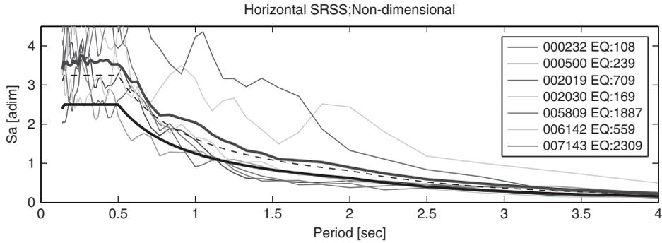
**FIGURE 12** Site class B. Example of horizontal non-dimensional set ( $\delta_H = 0.12$ ) featuring records from seven different earthquakes.
