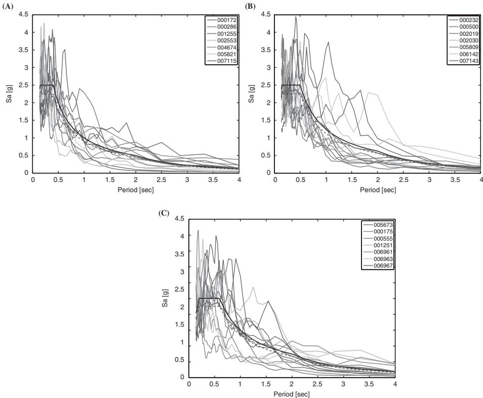
**FIGURE 16** Sets given in Figs. 11–13 recombined to take the average on all 14 horizontal components and compared to the code spectra.
