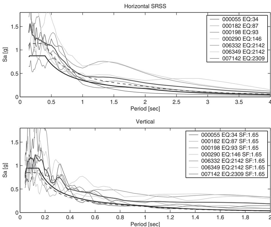
**FIGURE 2** Site class A – Zone 1. Set found having the minimum deviation of the average horizontal spectrum with respect to the target spectrum ( $\delta_H = 0.235$ ).
