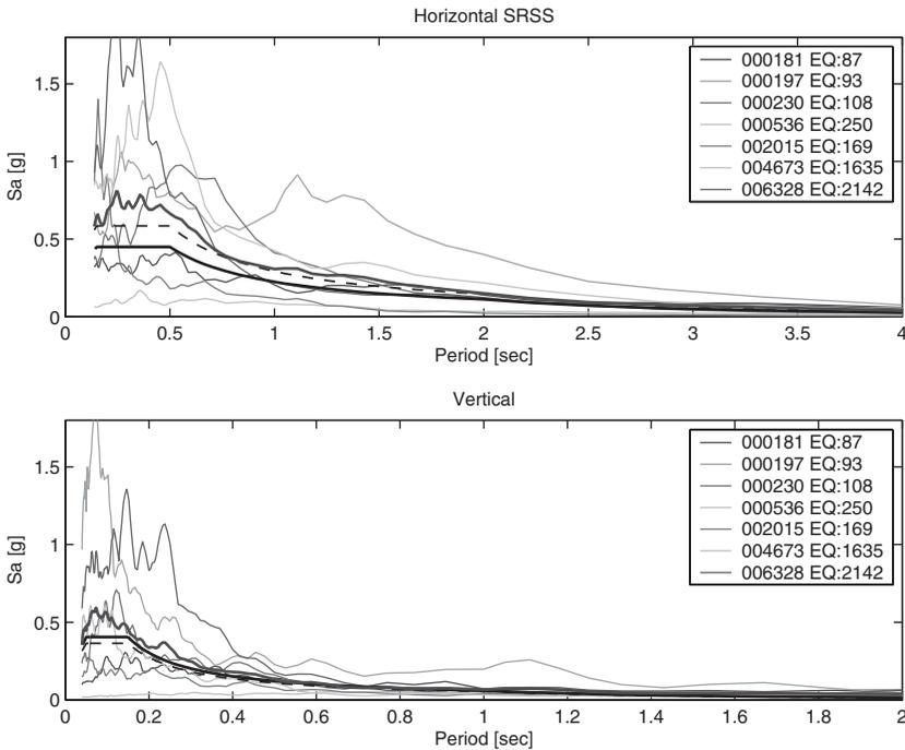
**FIGURE 7** Site class B – Zone 3. Set found having the minimum deviation of the average vertical spectrum from the target ( $\delta_V = 0.338$ ) and also featuring records from seven different earthquakes.
