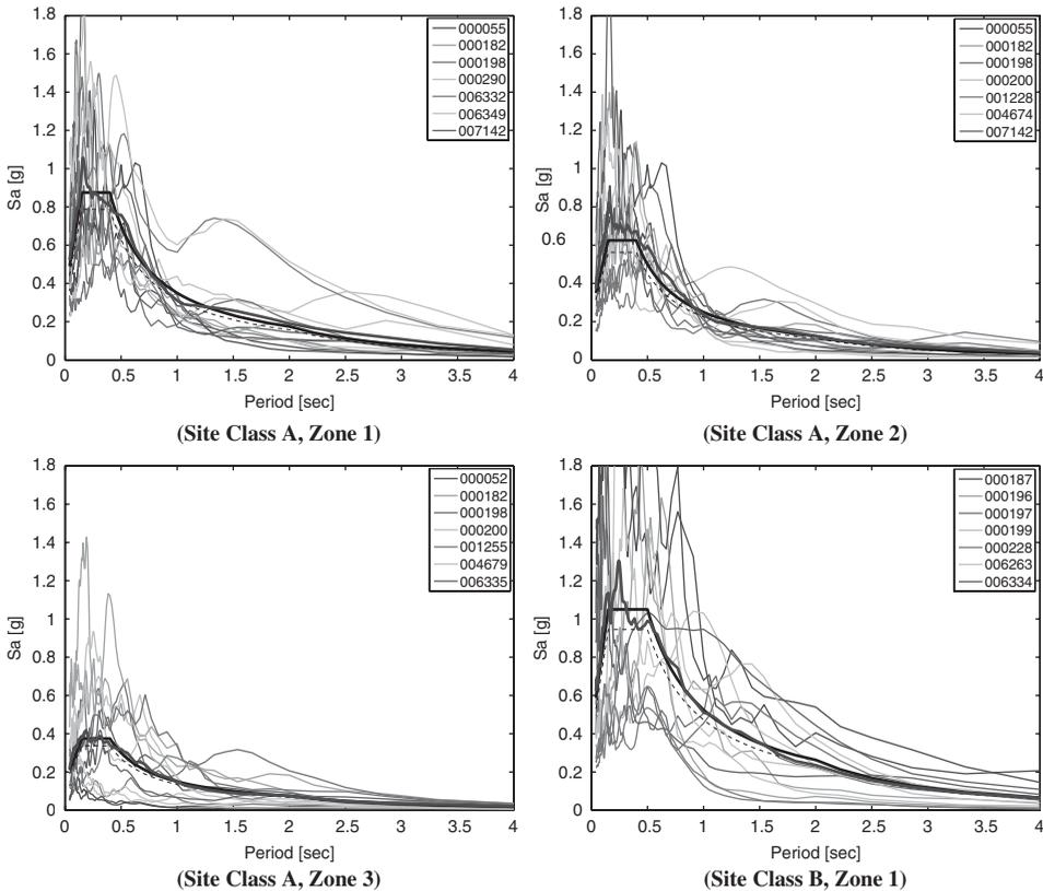
**FIGURE 14** Sets given in Figs. 2–5 recombined to take the average on all 14 horizontal components and compared to the code spectra.
