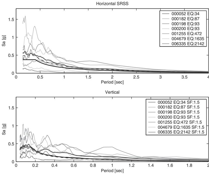
**FIGURE 4** Site class A – Zone 3. Set found having minimum individual deviation of horizontal and vertical spectra from their respective targets ( $\delta_{Hmax} = 1.336$ ;  $\delta_{Vmax} = 0.799$ ).
