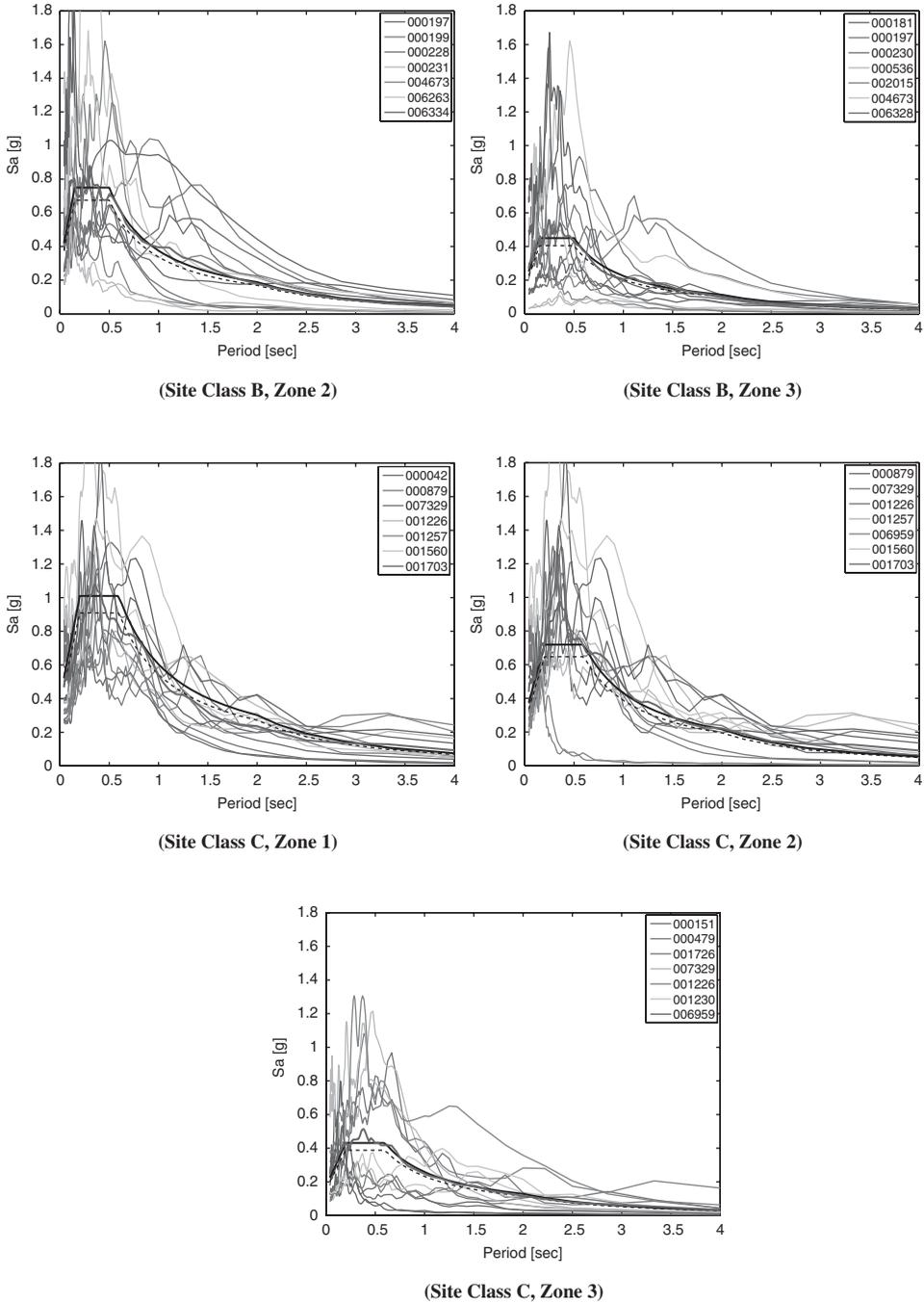
**FIGURE 15** Sets given in Figs. 6–10 recombined to take the average on all 14 horizontal components and compared to the code spectra.
