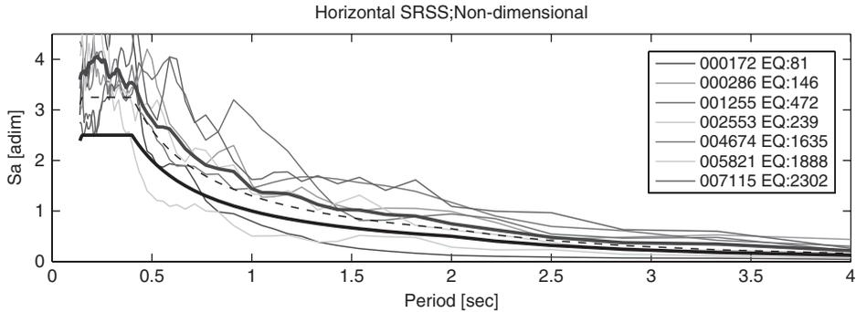
**FIGURE 11** Site class A. Example of horizontal non-dimensional set ( $\delta_H = 0.18$ ) featuring records from seven different earthquakes.
