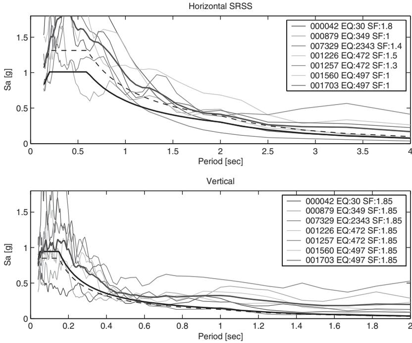
**FIGURE 8** Site class C – Zone 1. Set with minimum deviation of individual spectra from the horizontal target spectrum ( $\delta_{Hmax} = 0.525$ ), and minimum deviation of the vertical average spectrum from the target spectrum ( $\delta_V = 0.125$ ).
