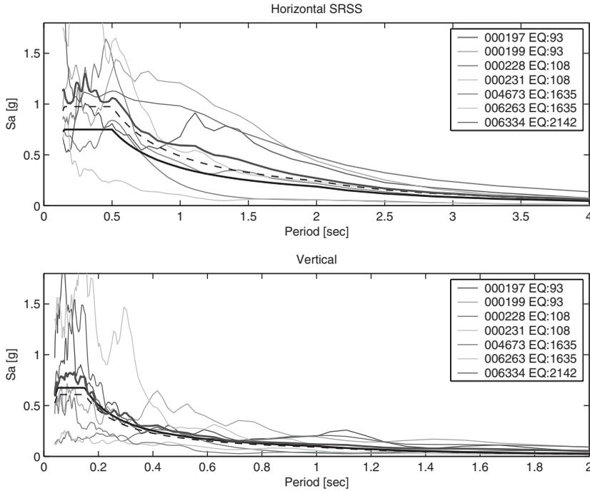
**FIGURE 6** Site class B – Zone 2. Set found having the minimum deviation of the average vertical spectrum from the target ( $\delta_V = 0.175$ ).
