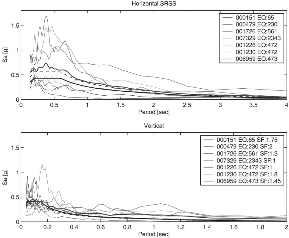
**FIGURE 10** Site class C – Zone 3. Set with minimum deviation of individual spectra from the horizontal and vertical target spectra ( $\delta_{Hmax} = 1.274$ ;  $\delta_{Vmax} = 1.163$ ) and minimum deviation of the average spectrum from the horizontal target spectrum ( $\delta_H = 0.147$ ).
