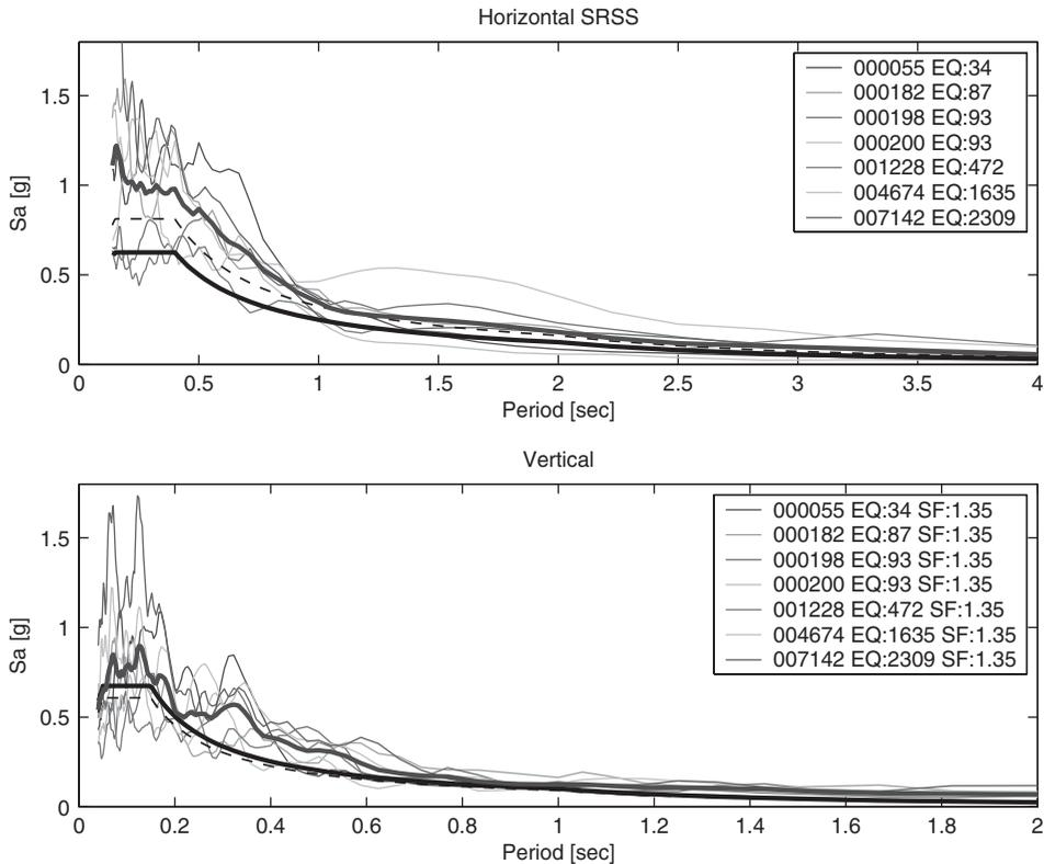
**FIGURE 3** Site class A – Zone 2. Set found having minimum deviation of individual horizontal and vertical spectra in from their respective targets ( $\delta_{Hmax} = 0.808$ ;  $\delta_{Vmax} = 0.513$ ), and also having minimum deviation of the vertical average spectrum with respect to the target ( $\delta_V = 0.231$ ).
