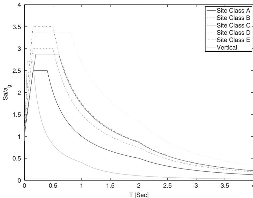
**FIGURE 1** EC8 horizontal and vertical type 1 spectral shapes.
