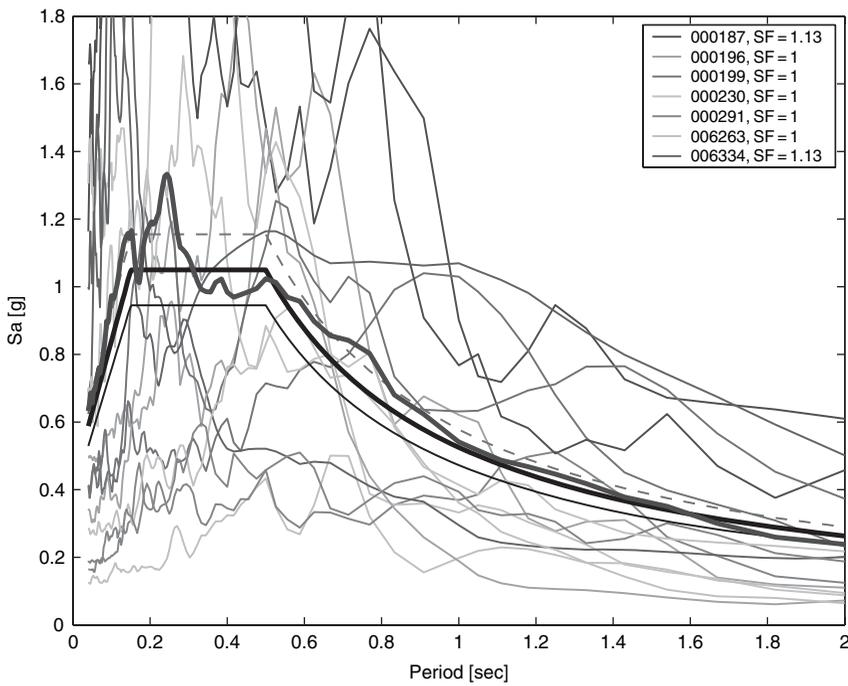
**FIGURE 8** Site class B – Zone 1. Set with minimum average deviation from target spectrum ( $\delta = 0.07$ ). SF is the individual scale factor.
