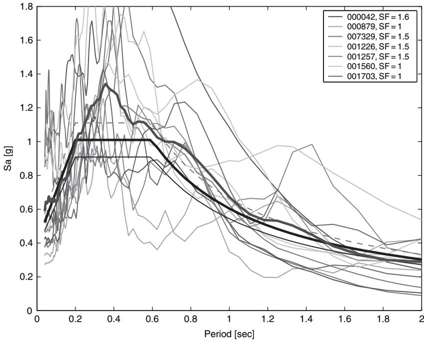
**FIGURE 11** Site class C – Zone 1. Set with minimum average deviation from target spectrum ( $\delta = 0.173$ ). SF is the individual scale factor.
