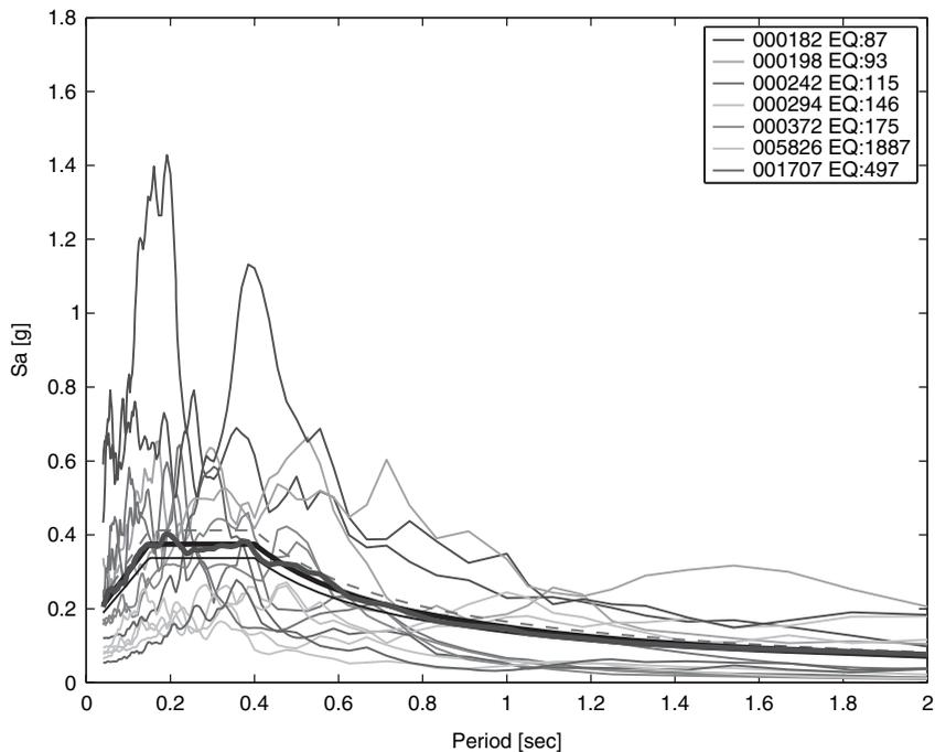
**FIGURE 3** Site class A – Zone 3. Set with minimum average deviation from the target spectrum ( $\delta = 0.041$ ) with records coming from seven different events.
