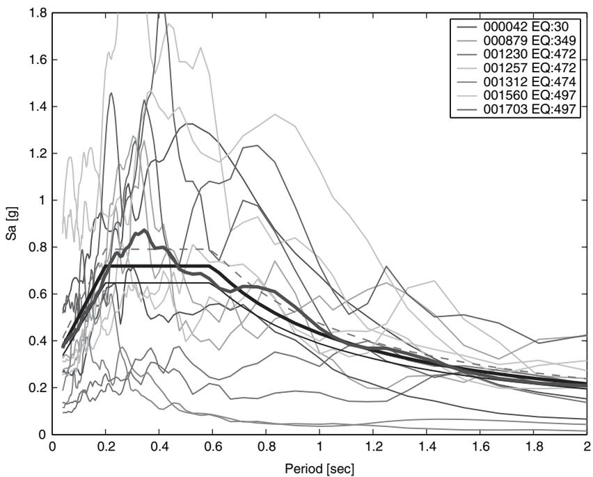
**FIGURE 10** Site class C – Zone 2. Set with minimum average deviation from target spectrum ( $\delta = 0.08$ ).
