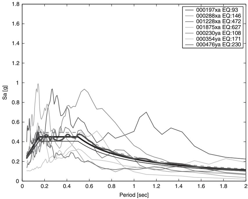
**FIGURE 15** Site class B – Zone 3. Set with minimum average deviation from target spectrum ( $\delta = 0.06$ ).
