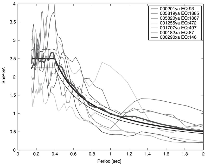
**FIGURE 22** Site class A – P-Type. Set with minimum average deviation from the target spectrum ( $\delta = 0.058$ ) with records coming from seven different events.
