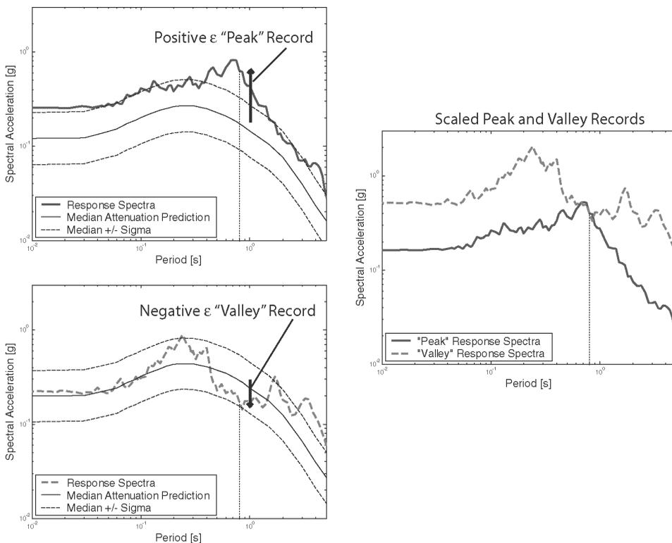
**FIGURE 1** Scaling a negative  $\epsilon$  record and a positive  $\epsilon$  record to the same spectral acceleration at the period of 0.8 s. Courtesy of Jack W. Baker; see Baker and Cornell [2005] for details.
