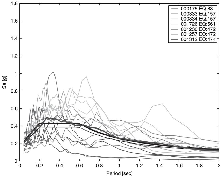
**FIGURE 9** Site class C – Zone 3. Set with minimum average deviation from the target spectrum ( $\delta = 0.07$ ) and minimum single-record deviation from the target ( $\delta_{\max} = 0.572$ ).
