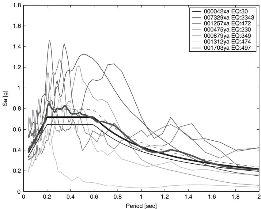
**FIGURE 19** Site class C – Zone 2. Set with minimum average deviation from the target spectrum ( $\delta = 0.08$ ) and minimum single-record deviation from the target ( $\delta_{\max} = 0.54$ ).
