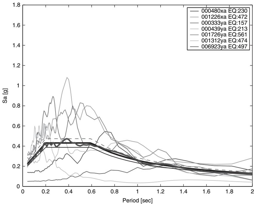
**FIGURE 18** Site class C – Zone 3. Set with minimum single-record deviation from the target spectrum ( $\delta_{\max} = 0.77$ ).
