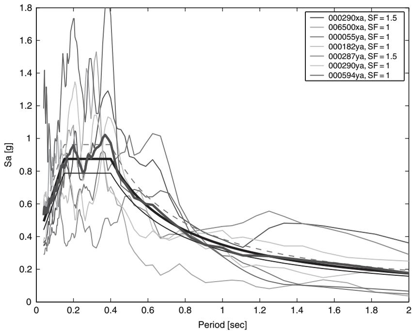
**FIGURE 14** Site class A – Zone 1. Set with minimum average deviation from target spectrum ( $\delta = 0.1$ ). SF is the individual scale factor.
