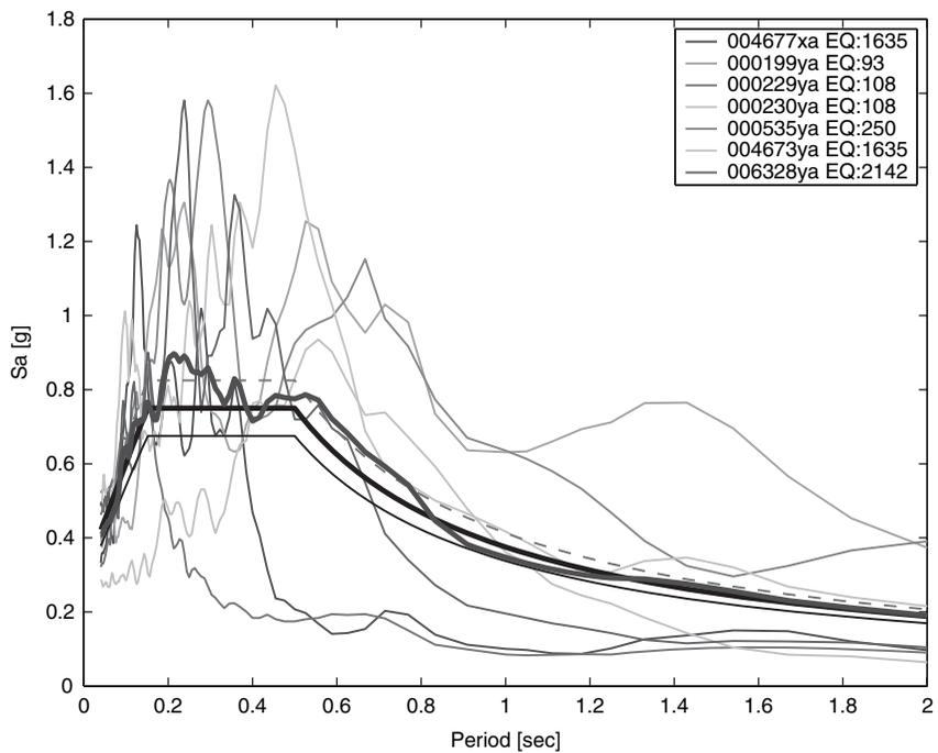
**FIGURE 16** Site class B – Zone 2. Set with minimum average deviation from the target spectrum ( $\delta = 0.09$ ) and minimum single-record deviation from the target ( $\delta_{\max} = 0.55$ ).
