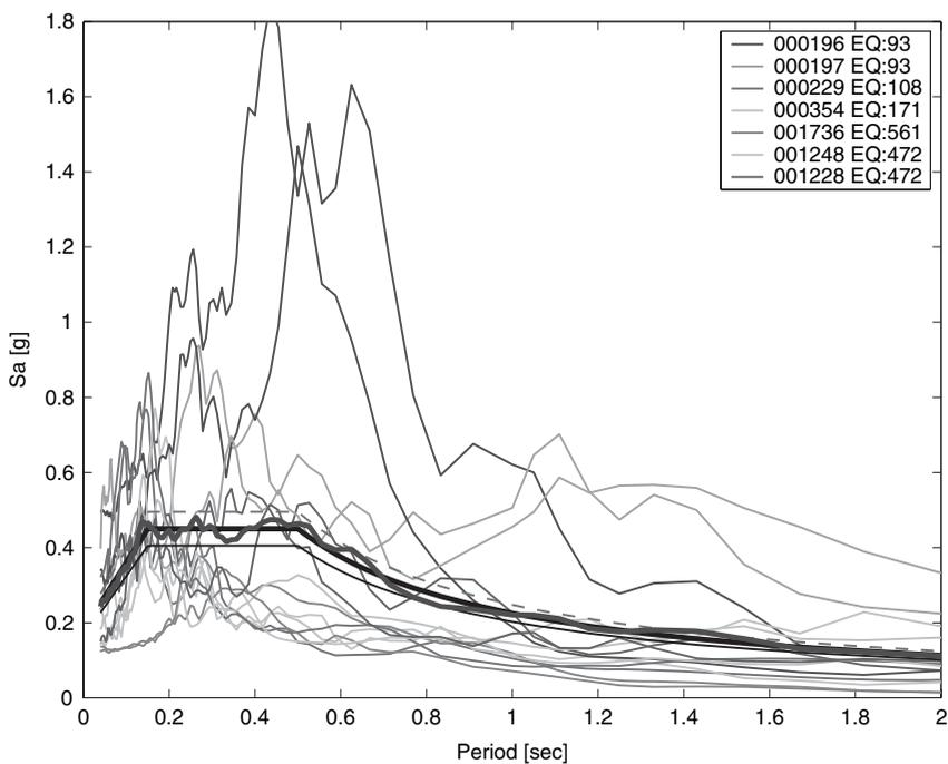
**FIGURE 6** Site class B – Zone 3. Set with minimum average deviation from the target spectrum ( $\delta = 0.04$ ) and minimum single-record deviation from the target ( $\delta_{\max} = 1.3$ ).
