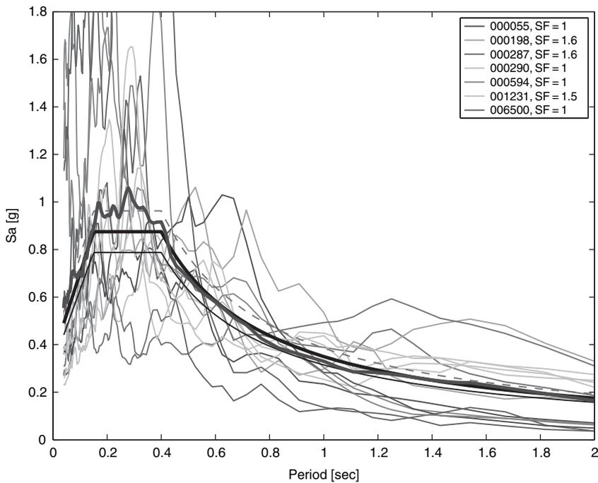
**FIGURE 5** Site class A – Zone 1. Set with minimum average deviation from target spectrum ( $\delta = 0.12$ ). SF is the individual scale factor.
