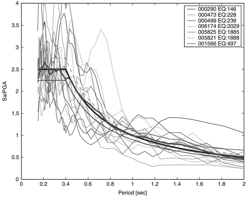
**FIGURE 21** Site class A – S-type. Set with minimum average deviation from the target spectrum ( $\delta = 0.047$ ) with records coming from seven different events.
