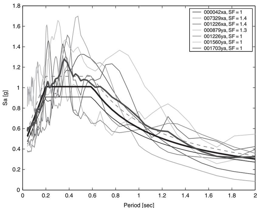
**FIGURE 20** Site class C – Zone 1. Set with minimum average deviation from the target spectrum ( $\delta = 0.11$ ) and minimum single-record deviation from the target ( $\delta_{\max} = 0.45$ ). SF is the individual scale factor.
