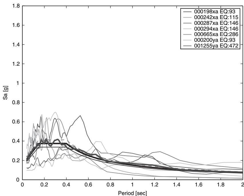
**FIGURE 12** Site class A – Zone 3. Set with minimum average deviation from the target spectrum ( $\delta = 0.07$ ) and minimum single-record deviation from the target ( $\delta_{\max} = 0.58$ ).
