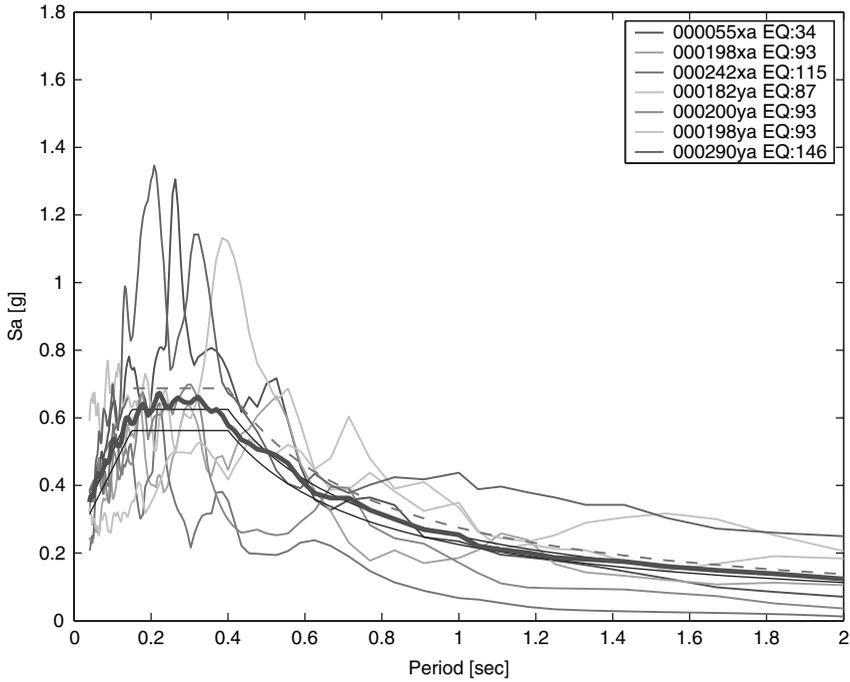
**FIGURE 13** Site class A – Zone 2. Set with minimum average deviation from the target spectrum ( $\delta = 0.04$ ) and minimum single-record deviation from the target ( $\delta_{\max} = 0.51$ ).
