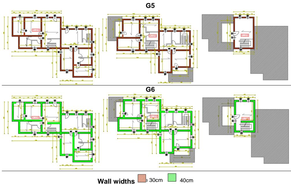
Figure 2.2.8 Plan views of configurations G5 and G6.
