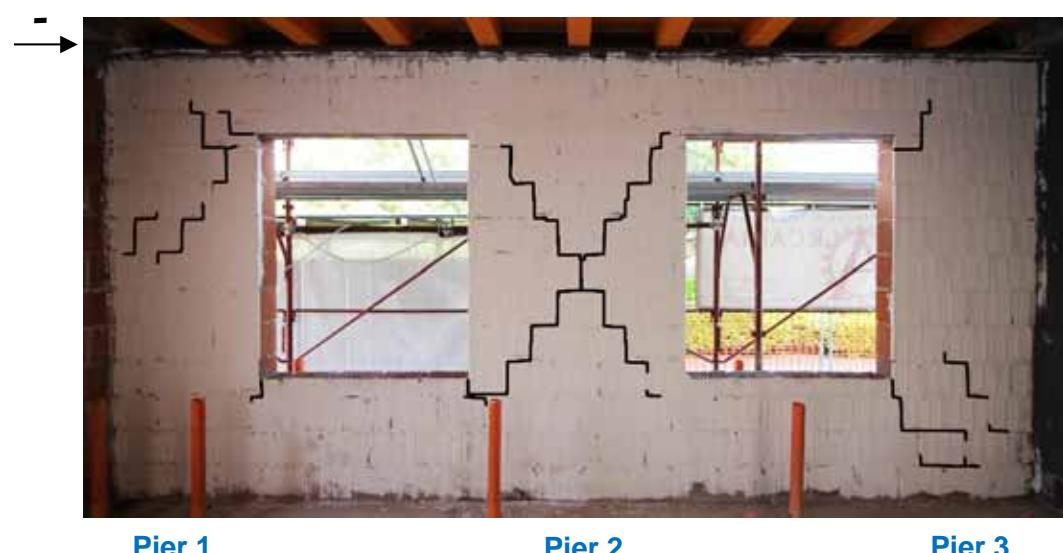
← + CRACK PATTERNS AT THE END OF EXPERIMENTAL TEST (inside view of East façade at ground floor)
