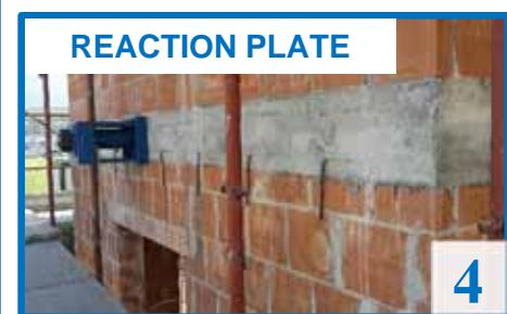
$$Drift (\%) = \frac{\delta_2}{h_2} = \frac{\frac{[(H2SW - BSW) + (H2SE - BSE)]}{2}}{h_2} = \frac{average\ top\ floor\ displacement}{height\ of\ 2nd\ floor\ horizontal\ load}$$
