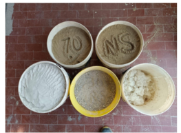
Composite mortar (Natural sand (NS), recycled sand (RS), NHL (mortar), chopped sheep wool fiber)
