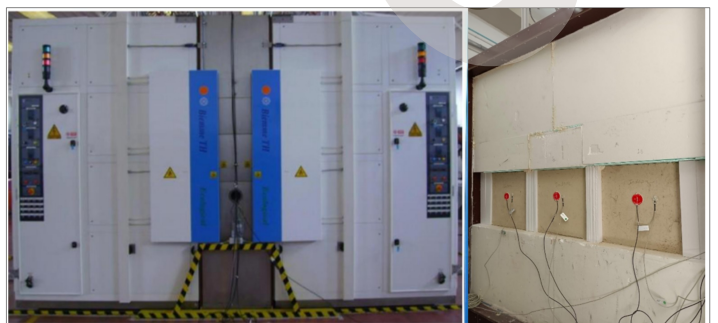
Thermal conductance test: (a) Climate chamber, and (b) masonry wall specimens placed at the central wall.
