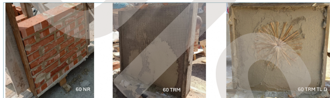
Some masonry walls: (a) Un-strengthened masonry wall, (b) masonry wall retrofitted with TRM system, and (c) masonry wall retrofitted with TRM, diatons and thermal layers.
