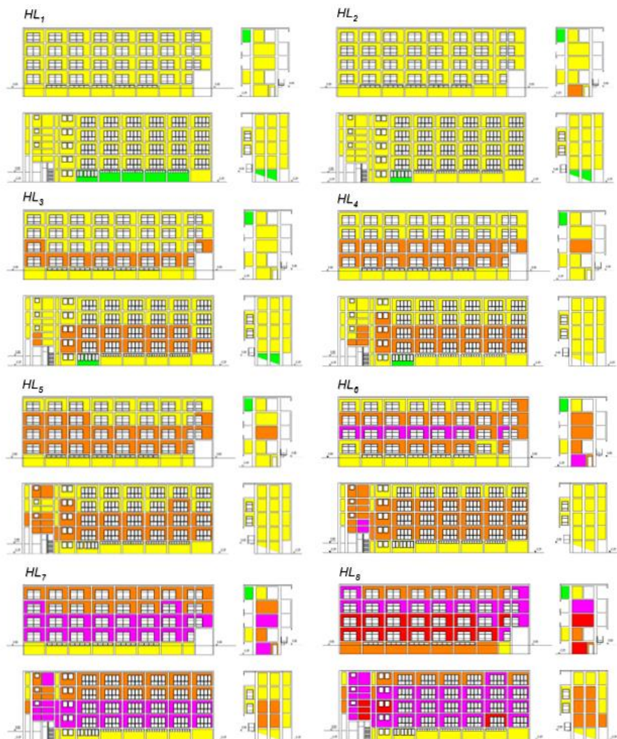
Figure 15. Colour representation of the state of all infills of the building at the eight hazard levels according to the chromatic scale of the backbone curve.
